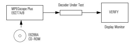
The E6288A CD–ROM contains 84 bit streams in the form of 204–byte MPEG–2 transport streams. You can load the streams onto the HP E6277A/B MPEGscope Plus to play them to the decoder under test. In most cases, the word "VERIFY" displays on the monitor if the decoder successfully passes the test. For further details on test results, refer to "Sarnoff Compliance Bitstreams for MPEG Video—User's Manual".
